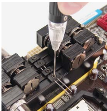
[Fig 23] Tighten the Wire Bracket Tabs
